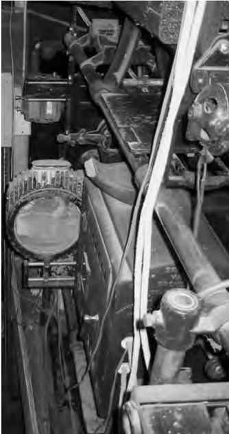
3. Heat sink tank located on a sliding rail. Shown here pulled out to the left side of the F7. An advertising slide for Gone with the Wind can be seen in the slide tray.
