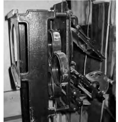
7. Front upright and projections assembly with turret lenses and pair of 45-degree mirrors. The slot for blending colour wheel is on the left.
