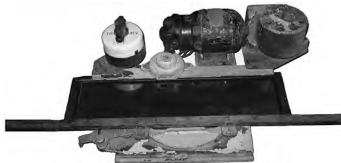
14. Electric panorama slide carrier with hand-painted Louvre panorama photographic slide
