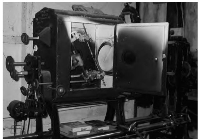
2. Lamphouse, showing carbon arc burner. The condenser lens is covered by the dowser shutter – used for fading. The automatic arc feeder mechanism can be seen at the back of the lantern below the normal manual arc controls.
