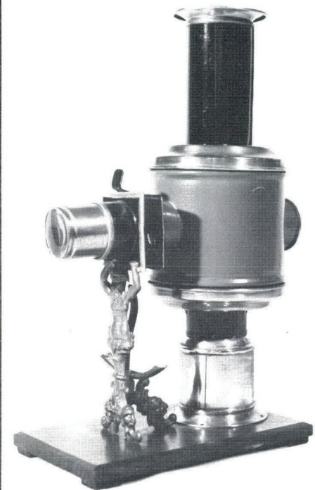
2. A Russian iron lantern by Butchers featuring the Stocks Patent paraffin lamp with a key operated telescopic chimney. The chimney acts in the same way as the glass on an oil lamp, creating an updraught which causes the flame to burn steadily, brightly, and continuously. The telescopic brass front is adjusted to approximately focus the slide on the screen with the rack and pinion on the lens used to make the final precise focus.
