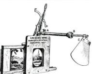
The effect obtained with it is good. For convenience in packing, it can be detached at a (see cut). By means of the nut B, the arm carrying the dissolver can be set at any required dis-tance to suit the focus of lens used.
