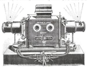
illustration, it will be seen that AA are objectives with prisms between the lenses; BB, slide carriers; c, illuminant; D, dissolving tap; E, roller curtain; FF, screws for rendering the discs co-incident.
