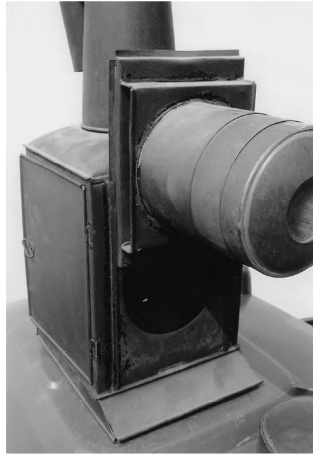
1. Martin Gilbert's bull's-eye lantern – detail of the vertically sliding detachable slide stage
